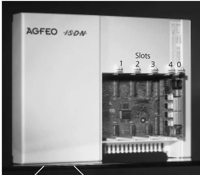
Figure 1: telephone system with detached cover
