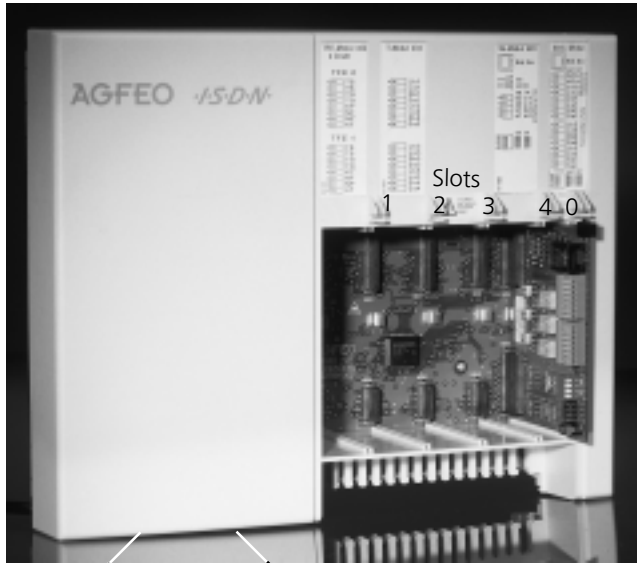
Figure 1: telephone system with detached cover
